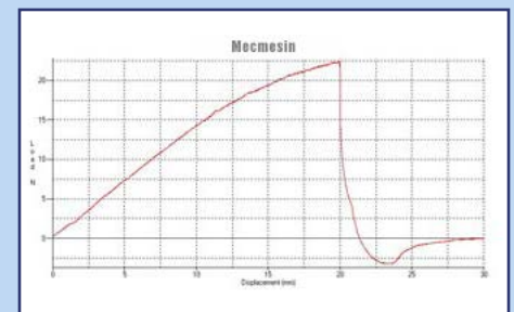
Back extrusion of confectionery frosting
